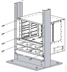
Rack Mounting the C300 Chassis
